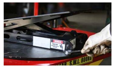
Table top attachments mount quickly and securely to the turntable with 4 x M12 bolts. The rotating turntable provides ease of movement when lining up components and bolt holes. (Pictured Above)
