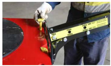
Changing front attachments can be done in moments; simply pull out the two yellow attachment pins, remove the existing attachment, slide the chosen attachment eyelets into the frame and replace the pins. (Pictured Above)
