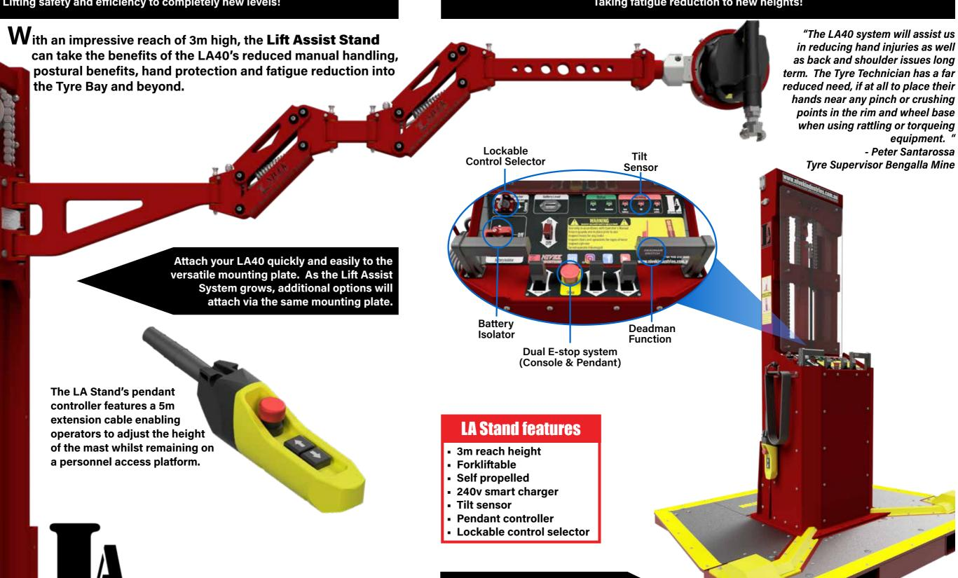
The LA Stand's base is forkliftable for moving from bay to bay and longer distances. It is also self propelled with a stand-on base for fine adjustment into position.
