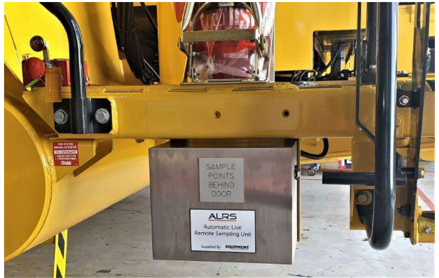
Installation of a 2-port sample station on Komatsu 930E dump truck
