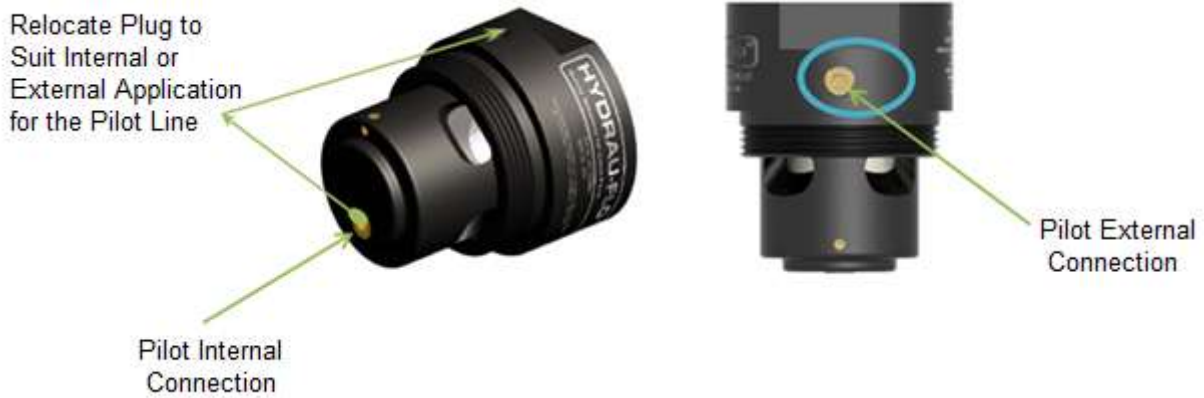
Figure 3-5: Converting External Pilot Line to an Internal Line
